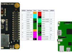
Now connect the your carrier boa second Pi's GPIO with three jumper wires (female to female):
