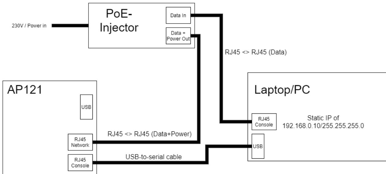
4. Open the Device Manager and select Ports, there you should see an interface like COM1 or COM3. Select this interface in PuTTY as it is your serial cable to the AP.
